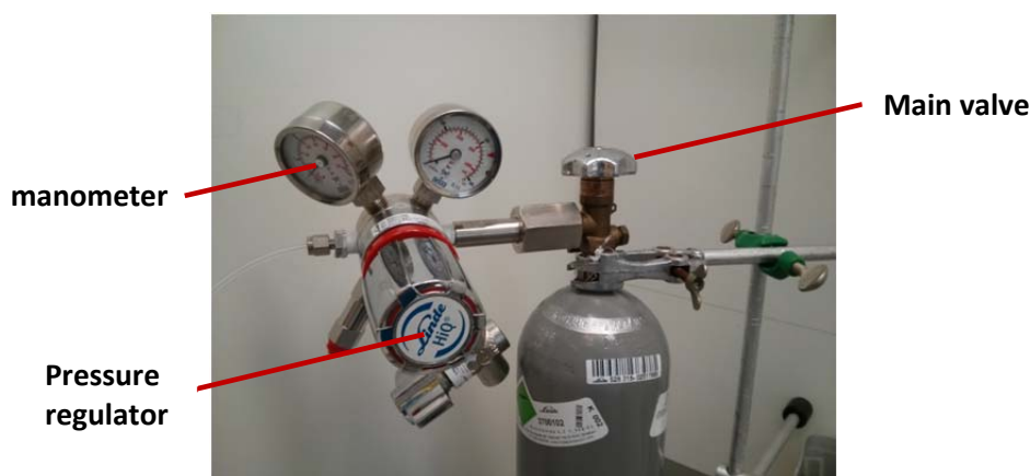
Figure 3.3: Pressure regulation from the gas cylinder.
