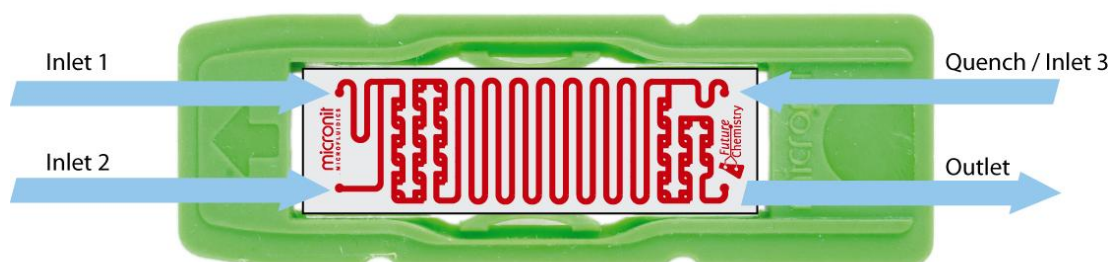
Figure 1: Schematic view Basic Quench Microreactor channel lay-out
